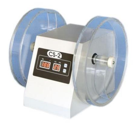
CS-1/2/3 Series Tablet Friability Tester Series are the latest development and production of our company, which is the requisite instrument in detecting the friability and abrasion of tablets. The design and technical specifications of this tester reached or surpassed the advanced level of its kind of instrument in the world. All our lab instruments are manufactured in conformance to USP Specifications and Codes.
